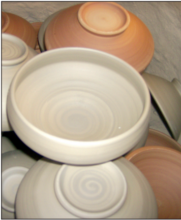
■ Fig. 11 Test 2 (left). Unfired pottery stacked in the kiln. ■ Fig. 12 Test 2 (middle). The same bowls after the cooling. Note different shades of grey on the topmost ones. ■ Fig. 13 Test 2 (right). Fired bowls after the extraction from the firing chamber.
