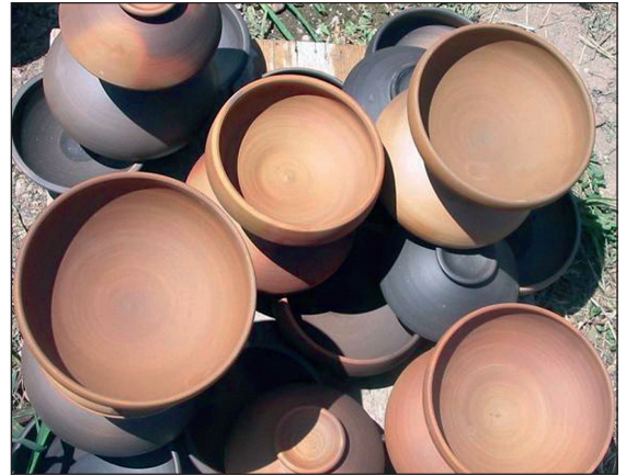
■ Fig. 11 Test 2 (left). Unfired pottery stacked in the kiln. ■ Fig. 12 Test 2 (middle). The same bowls after the cooling. Note different shades of grey on the topmost ones. ■ Fig. 13 Test 2 (right). Fired bowls after the extraction from the firing chamber.
