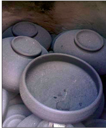
■ Fig. 11 Test 2 (left). Unfired pottery stacked in the kiln. ■ Fig. 12 Test 2 (middle). The same bowls after the cooling. Note different shades of grey on the topmost ones. ■ Fig. 13 Test 2 (right). Fired bowls after the extraction from the firing chamber.
