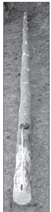
■ Fig. 9 Wooden pile cut for the experiment
