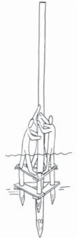
■ Fig. 15b Schematic illustration of the beginning of the experiment (three people standing on the movable structure, ready to begin driving the pile in the lake marl – the lake water level is about as high as the structure) (Drawing: B. Pollmann)
