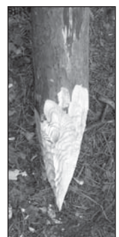
■ Fig. 10 Pointed end of the wooden pile used in the experiment
