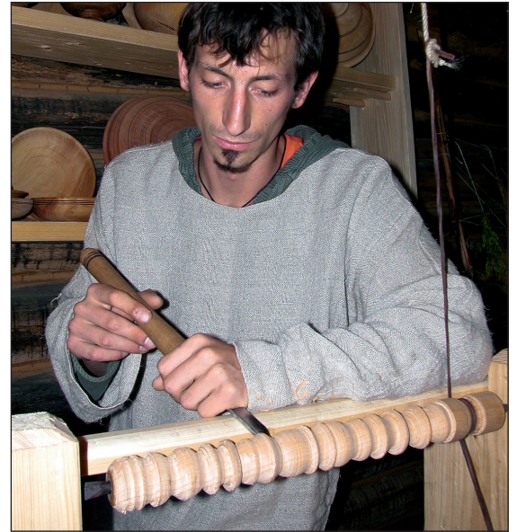
■ Fig. 6 In the woodworkers house a wooden lathe machine was built to turn wooden vessels like plates, dishes and bowls.
