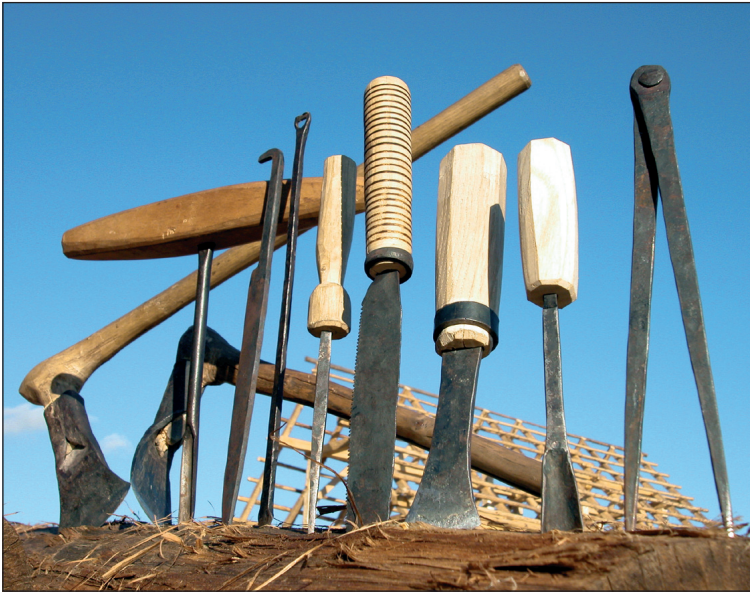
■ Fig. 4 The iron reconstructions of period tools which we used during the construction work: axes, adzes, drawing knife, knives, chisels, spoon drills, awls, etc.
