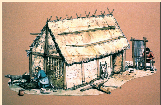
■ Fig. 6 The walls of Anglo-Saxon houses were made with wattle (woven branches) and daub (clay).
