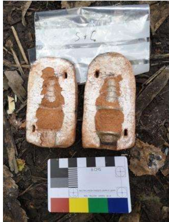
Figure 26 The sand-clay mould after casting. (Photo taken by Author: 2019).
