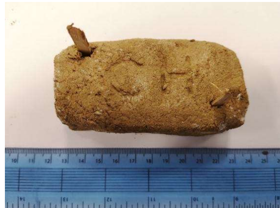
Figure 13 The chapped rice hull mould had been dried for one day (Photo taken by Author: 2019).
