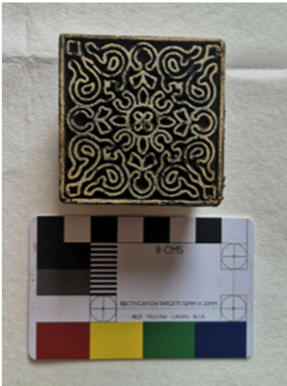
Figure 6 The stamp used to make patterns on the surface of moulds (Photo taken by Author: 2019).
