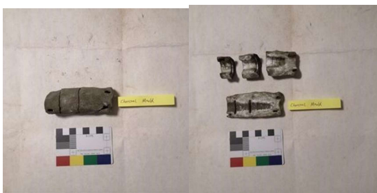
Figure 29 The charcoal mould broken during drying (Photo taken by Author: 2019).
