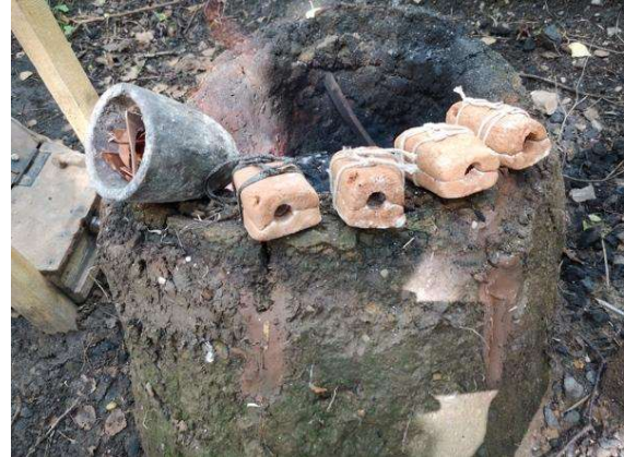
Figure 22 The pouring gate of moulds is oriented away from the fire (Photo taken by Author: 2019).
