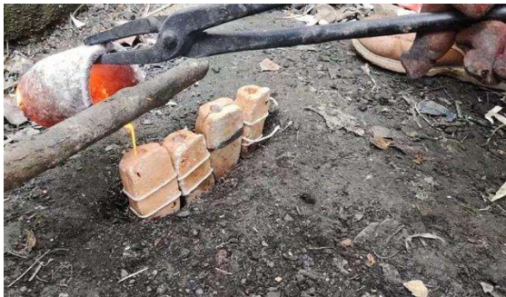
Figure 25 The molten bronze was poured into moulds (Photo taken by Author: 2019).
