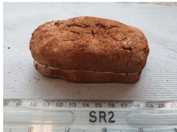
Figure 19 The baking sand-clay mould (Photo taken by Author: 2019).
