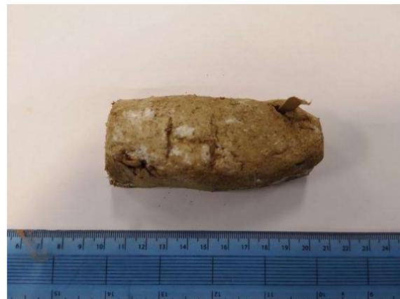
Figure 13 The chapped rice hull mould had been dried for one day (Photo taken by Author: 2019).
