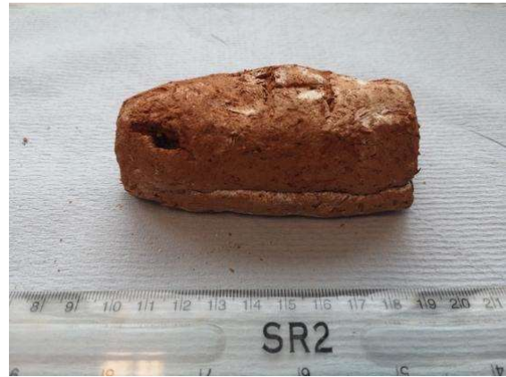
Figure 18 The baking rice hull mould (Photo taken by Author: 2019).
