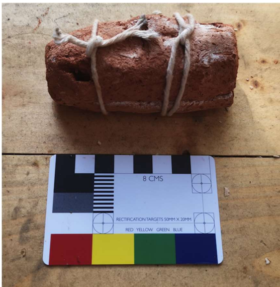
Figure 21 The rice hull mould tied with a rope (Photo taken by Author: 2019).
