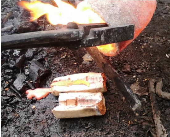
Figure 34 The molten bronze is poured on a half of wood ash mould (Photo taken by Author: 2019).
