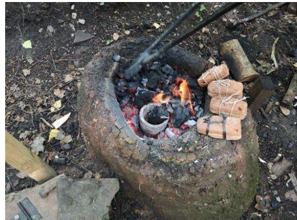
Figure 23 A crucible was inserted into the bowl hearth (Photo taken by Author: 2019).
