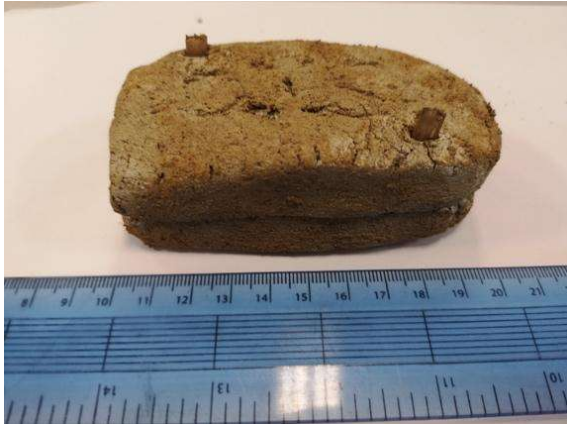
Figure 15 The sand-clay mould had been dried for one day (Photo taken by Author: 2019).
