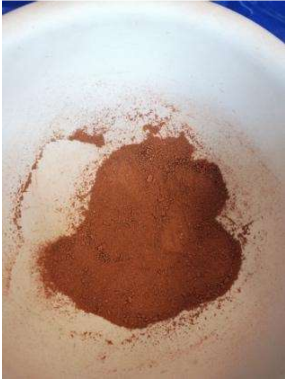
Figure 28 A part of the ash (rice hull) mould was grinded to grog (Photo taken by Author: 2019).
