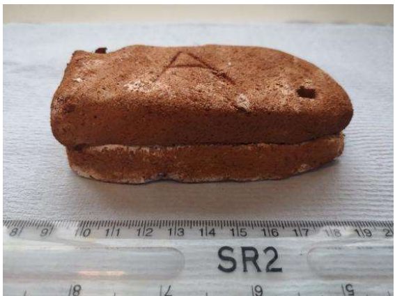
Figure 16 The baking ash (rice hull) mould (Photo taken by Author: 2019).
